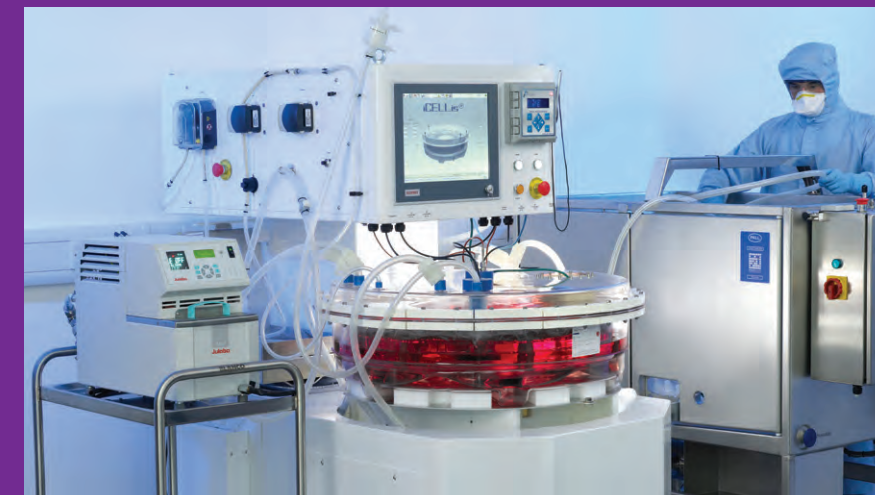
FIGURE 1 The new iCELLis 500 bioreactor from Pall can in many cases overcome the need to scale-out plasticware processes due to its larger capacity. PHOTO COURTESY OF PALL LIFE SCIENCES
